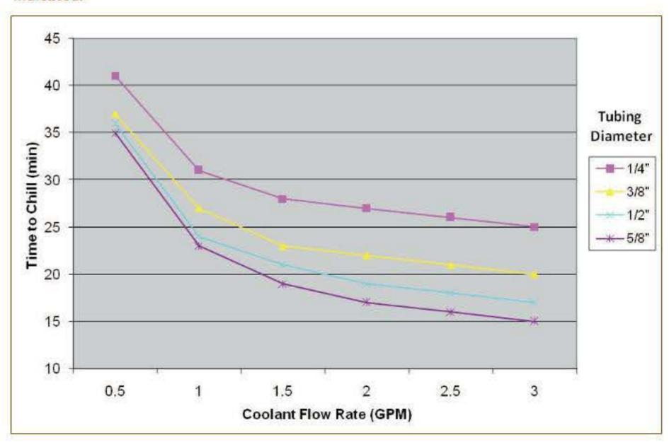
FIGURE 2. CHILLING TIME BY LENGTH AND TUBING DIAMETER. This figure provides the estimated time to chill 5 gallons of 13 °P wort from 200° F to 80° F using 70° F coolant water flowing at 2.5 gpm with a chiller sized as indicated.
