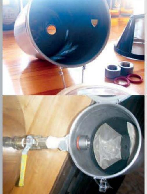
gravity flow the wort (5 gallons) through about 3 ounces of hops at a time, before draining out the bottom and into the fermenter.
